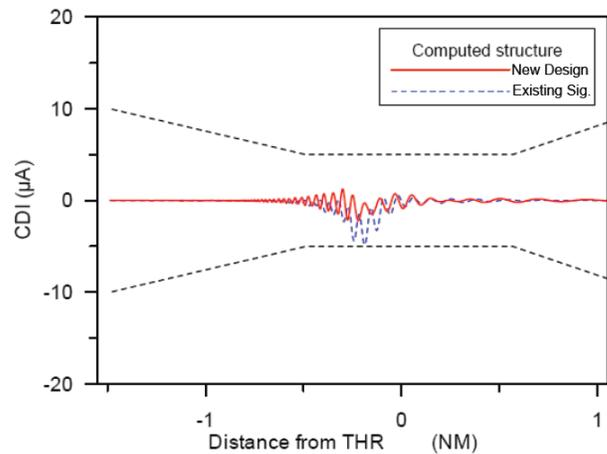
**Figure 2: Modeled Reduction in Centerline Distortion**
