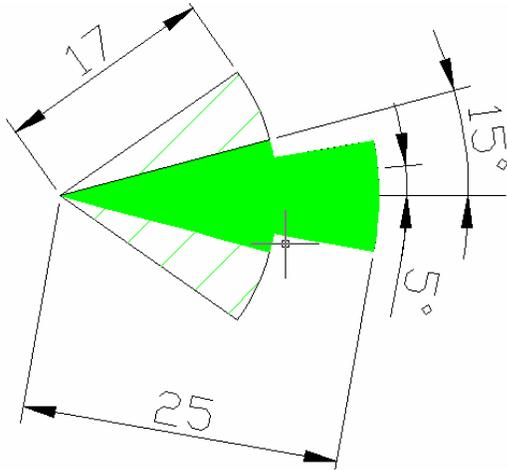
**Figure 8: Proposed ILS Coverage Requirements (Ranges in NM)**
