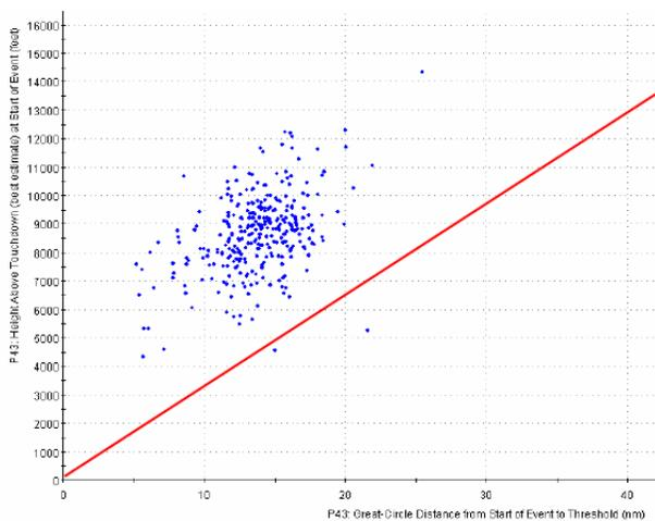
**Figure 9: Vertical Distribution of High Workload T-Approaches (Height Above Touchdown [ft] vs. Distance to Threshold [NM])**
