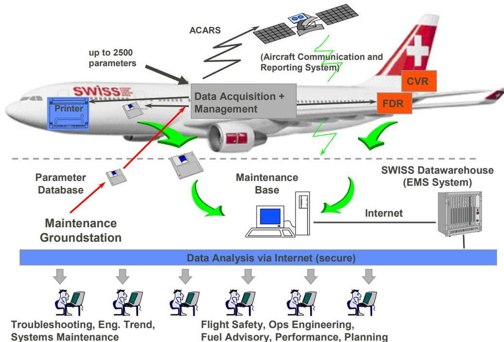
**Figure 5: EMS is the ground based core part of the Aircraft Data Acquisition System (ADAS)**
