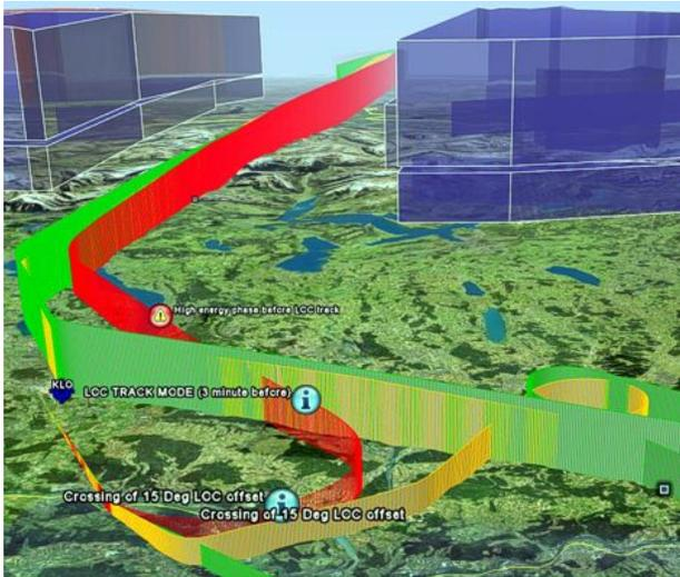
**Figure 6: Visualization of ILS Approaches with Different Workload Levels**
